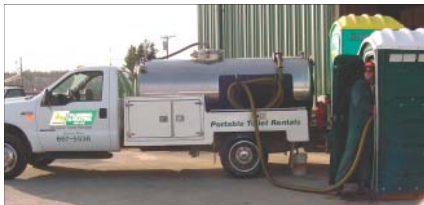
Craig Clement services a portable restroom with Ray Plumbing's 2000 Ford 550 Super Duty with Coleman PSB950 body (stainless steel tank, fiberglass body, 600-gallon waste tank, 270-gallon heated wash water tank, 80-gallon heated rinse water capacity).
